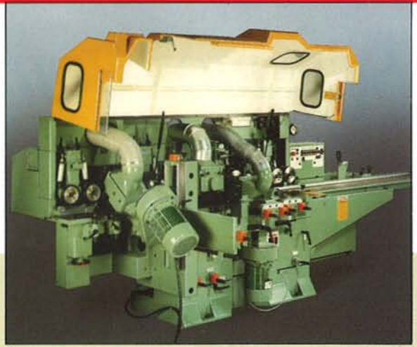
△ GD5 from outfeed end with cover open showing 4 position Universal Head.
